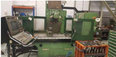
Fresadora vertical 1700 mm. ZAYER 1700 AF3 Ref: TF-002
