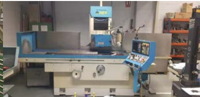
Rectificadora superficies planas 1000x500 mm. GER S-100/50 Ref: TF-001
